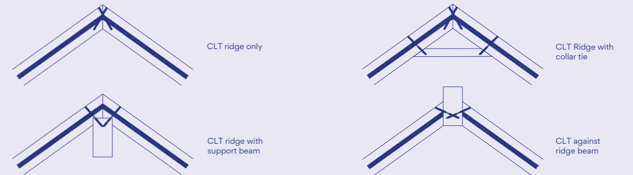
Roof ridge connection
